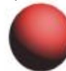
Dia.0,5mm Uranium Dioxide Fuel
